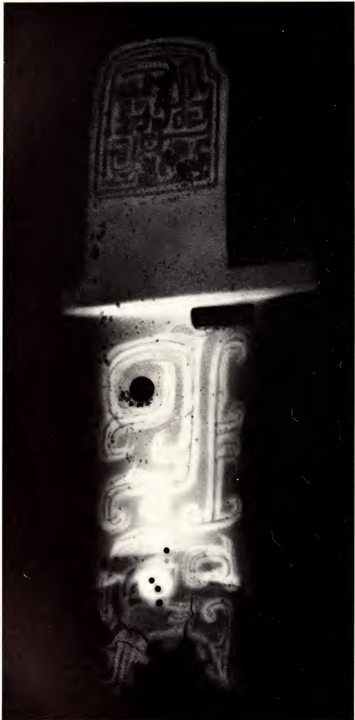
FIG. 11.—34.11. Radiograph of the bronze dagger axe. The radiograph shows that the iron rust deposit at the point end conceals an open dragon's mouth and that the bronze blade was cast-on to the point which had been shaped in the form of a key so that bronze and iron are securely locked together. Radiograph taken at 250 Kv, 10 Ma, distance from target 183 cm.; developed in Eastman Kodak Microdol developer. Courtesy, U.S. Naval Ordnance Laboratory.
